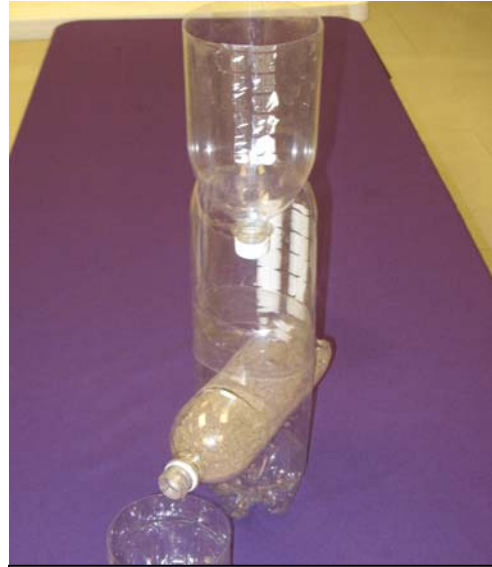
Complete assembly includes 3 two-liter bottles and 1 one-liter bottle.
