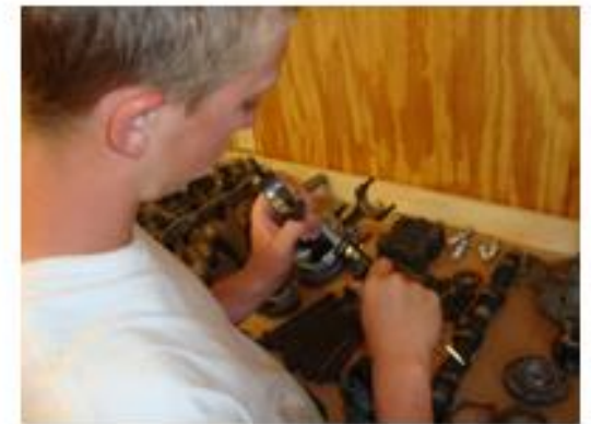
Measuring piston rods on the Toyota engine.
